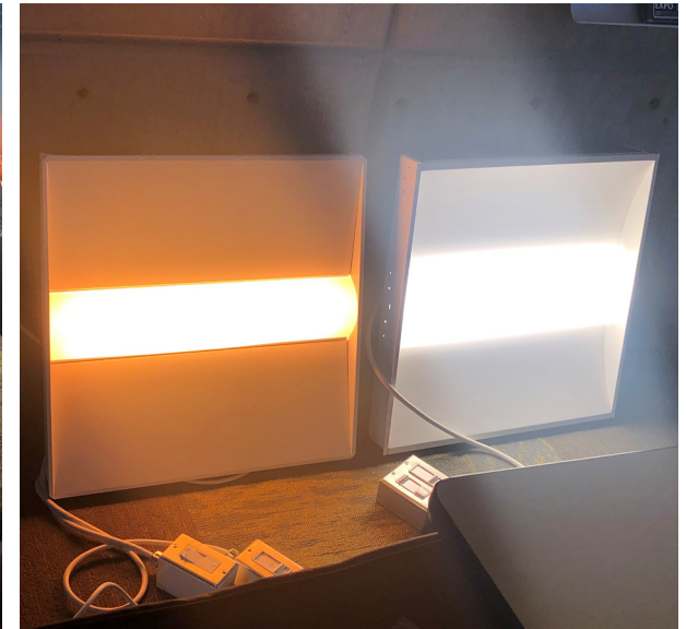
Bottom: evaluating sample fixtures to confirm desired temperature range and operation
